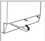
3. using a screwdriver, remove the cover panel on the lower front part of the washer-dryer (see figure).
